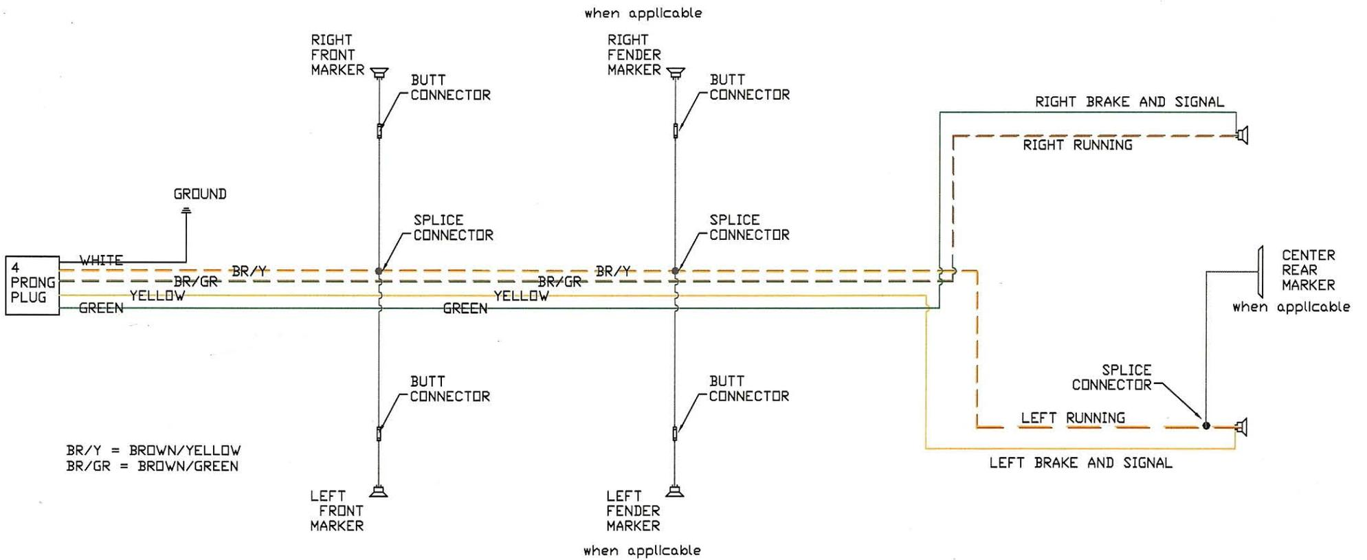
Note: To convert the 5 wire harness on the Teske trailer to a 4 prong replacement plug, combine the brown/green and brown/yellow wires into the slot next to the white ground wire.
